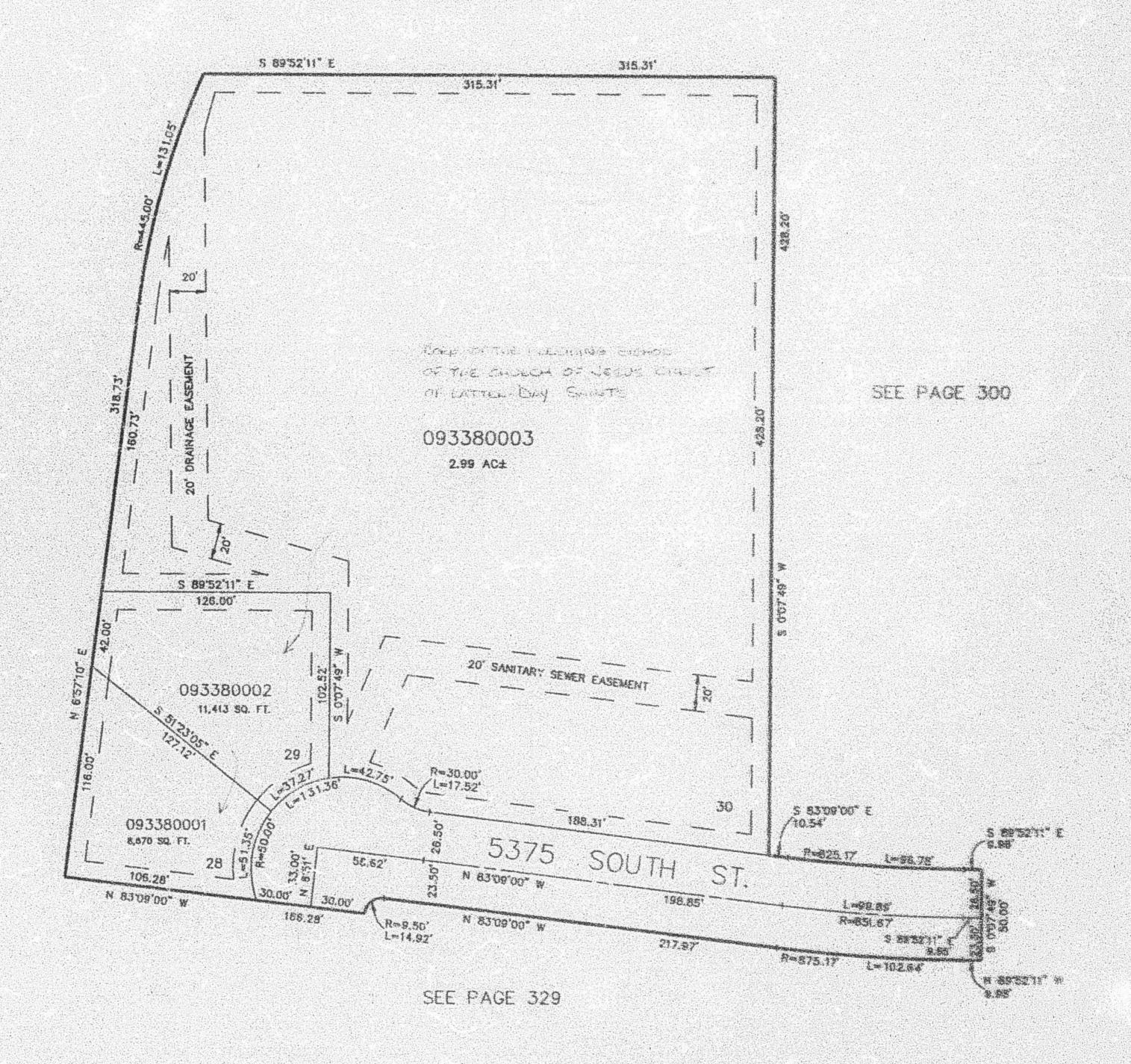
TO UTBUTY & DRAINAGE EASEMENTS EACH SIDE OF PROPERTY LINES AS INDICATED BY DASHED LINES EXCEPT AS OTHERWISE SHOWN.
